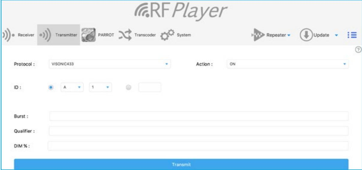
The screenshot shows the RF Player web interface for the SENDER configuration. The top navigation bar includes 'Receiver', 'Transmitter', 'PARROT', 'Transcoder', 'System', 'Repeater', and 'Update'. The main configuration area has 'Protocol' set to 'VISIONIC433' and 'Action' set to 'ON'. Below these are fields for 'ID' (with radio buttons for 'A' and '1'), 'Burst', 'Qualifier', and 'DIM%'. A blue 'Transmit' button is at the bottom.
